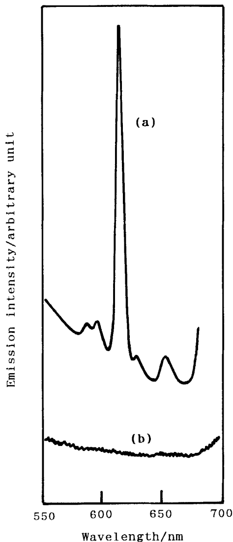
Figure 4 Fluorescence spectra of mononuclear Eu(III) (a) and heteronuclear Ni(II)-Eu(III) (b) complexes in DMF. The concentration of each complex is 2.5 \times 10^{-4} \text{ mol dm}^{-3} ; exciting wavelength is 394 nm; slit widths of excitation and emission sides are 20 and 5 nm, respectively; ordinate scales are \times 32 for (a) and \times 1024 (b).
